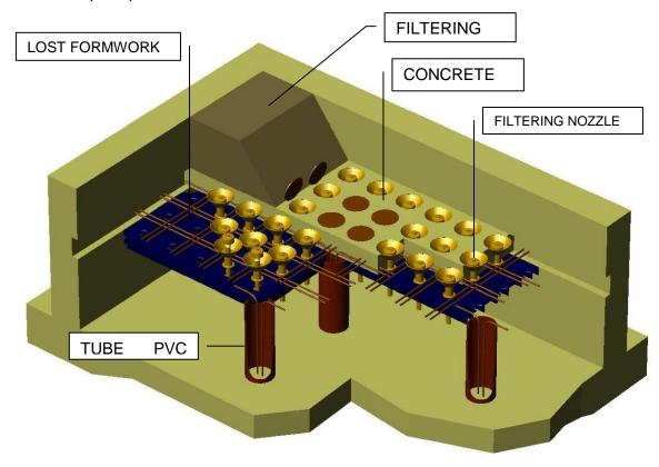
A filter with a MONOLITHIC CONCRETE SLAB (FALSE CONCRETE BOTTOM) has exactly the same working characteristics than a conventional filter (filtration velocity / backwash air / backwash water / highness / materials, types and density of filtering nozzles)
